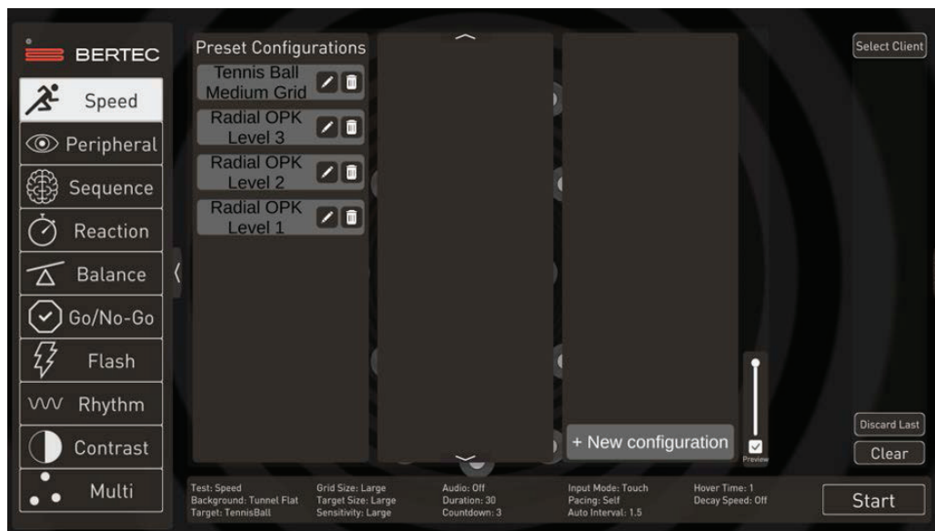
Figure 16: Preset configurations menu. To add a new preset, select the +New configuration button.
